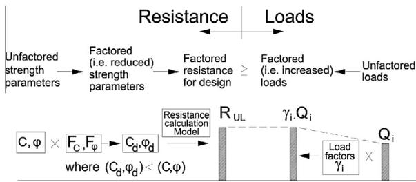
**Fig. 1** Schematic diagram for the concept of factored strength approach [9].
