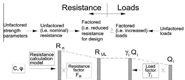
**Fig. 2** Schematic diagram for the concept of factored resistance approach [9].
