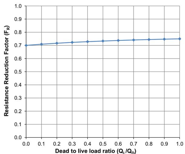
Fig. 4 Relation between  $F_R$  and  $Q_L/Q_D$  ratio for the empirical load-settlement relationship design method of axially loaded large diameter bored pile and static pile load test design method at  $FS_g$  equals 2.0.
