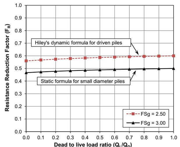
Fig. 3 Relation between calibrated  $F_R$  and  $Q_L/Q_D$  ratio for static and dynamic formula design methods adopted in the ECP-202 (2001).
