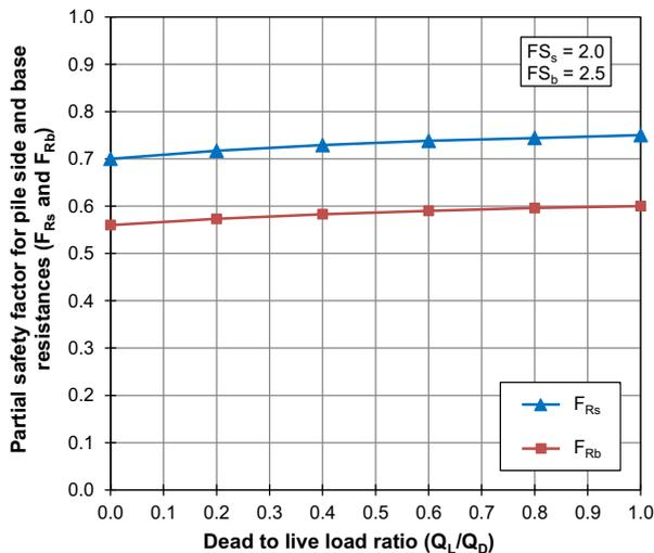
Fig. 6 Variation of  $Q_L/Q_D$  with  $F_{Rb}$  and  $F_{Rs}$  of the intersection point for SPT-based driven piles.
