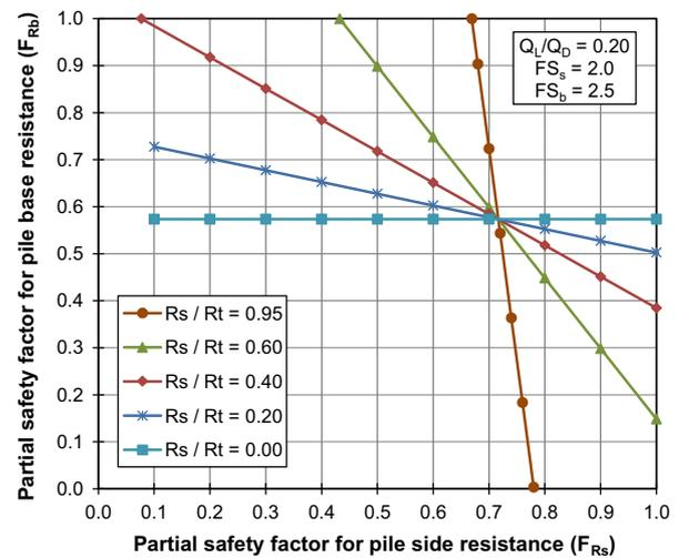
Fig. 5 Calibrated  $F_{R_s}$  and  $F_{R_b}$  with respect to the skin friction share for SPT-based driven piles.
